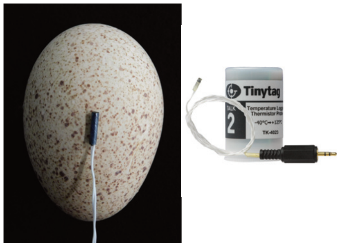
Figure 14. Correct attachment of data logger to the shell
