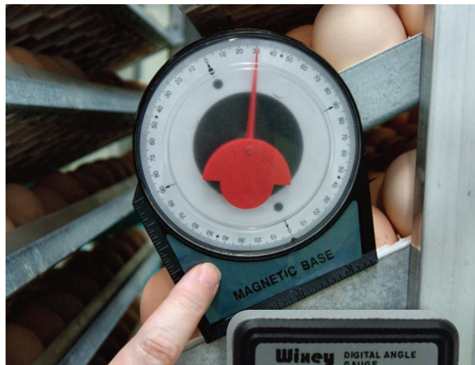
Figure 21a. Angle meter Figure 21b. Digital angle gauge. In both pictures the turning angle is too low, at around 30 degrees
