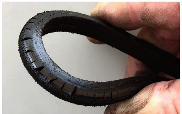
Figure 77. Worn fan belt
